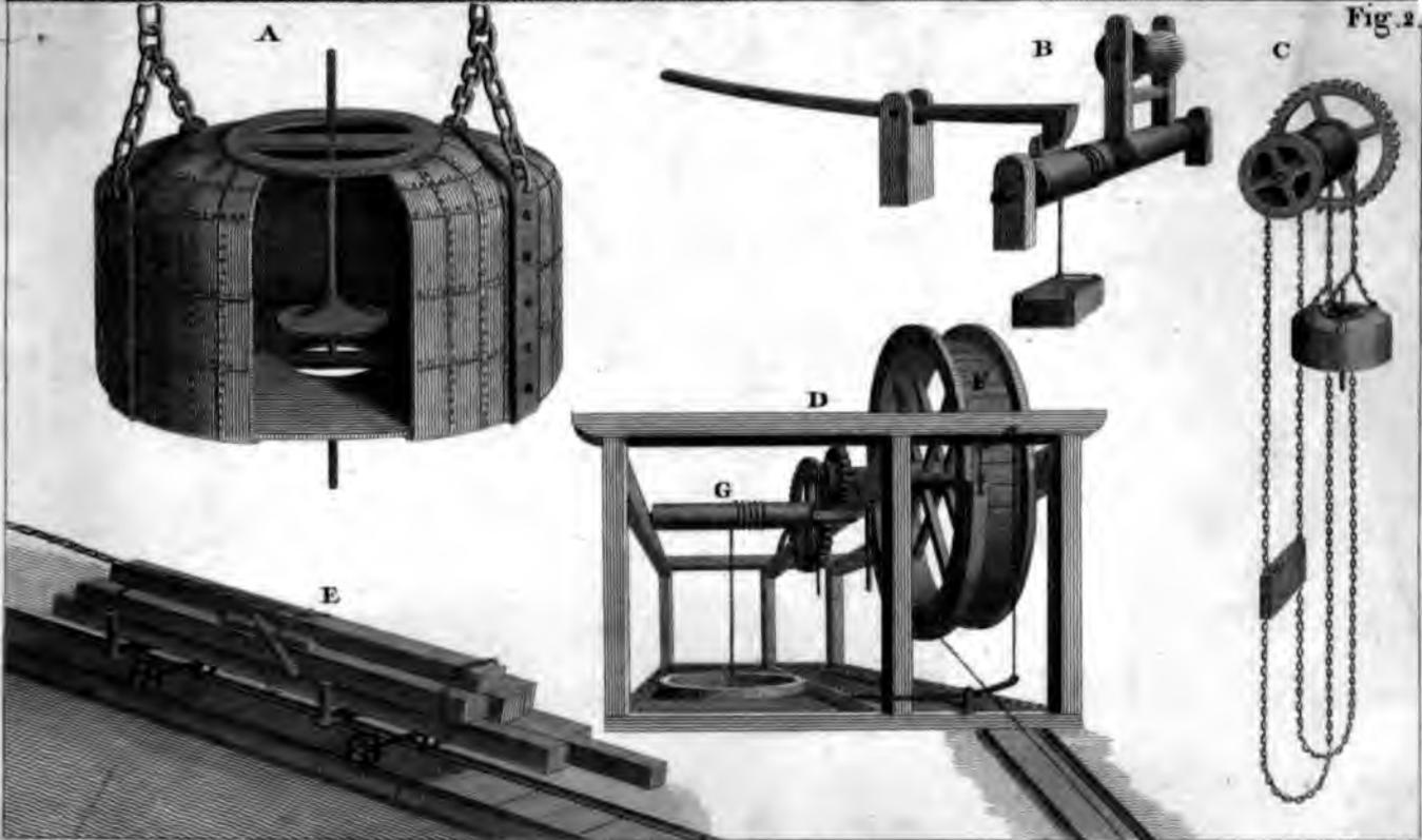
Fig. 1. the Cast off book, which Separates from the Leading Chains on the Boat entering the Various Levels. Also the Spined wheel with teeth to prevent the Chain Slipping.
